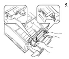
. Before closing the **front cover**, secure the **drum unit** into place by applying pressure at its top where the "**Press**" label is affixed. The **drum unit** will lock into place when it has been correctly inserted into the printer.
