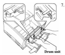
. Once the **image transfer roller unit** has been installed, secure the **drum unit** into place by applying pressure at its top where the "**Press**" label is affixed. The **drum unit** will lock into place when it has been correctly inserted into the printer.
