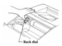
12. When installing the cartridge, hold the rack dial with your hand to prevent the rack from rotating.
