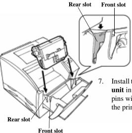
Install the image transfer belt unit in the printer, aligning its pins with the rear slots inside the printer's frame.
