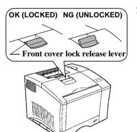
21. Make sure that the **front cover** is completely closed.
