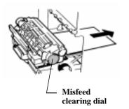
5. While turning the **misfeed** clearing dial of the fusing unit counterclockwise, pull out the paper from the **fusing** unit.
