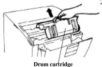
2. Holding the grip, pull out the drum cartridge.
