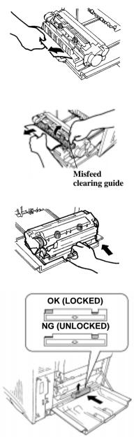
6. Pull out the paper from the fusing unit.
