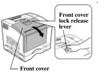
7. Grasp and pull down the **front** cover lock release lever to swing open the **front cover**.
