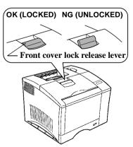
18. Make sure that the **front cover** is completely closed.
