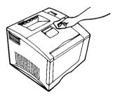
1. Using a soft cloth and a mild dishwashing detergent, wipe the outside of the printer.
