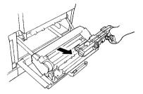
16. Loosen both of the **oiling** roller's installation screws.
