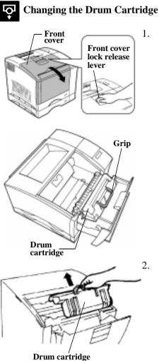
Grasp and pull down the front cover lock release lever and swing open the **front cover**.
