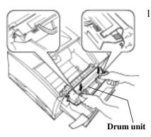
16. Once the toner cartridge has been installed, secure the drum unit into place by applying pressure at its top where the "Press" label is affixed. The drum unit will lock into place when it has been correctly inserted into the printer.
