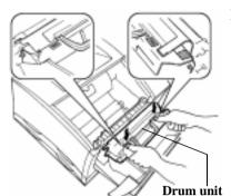
15. APPLY PRESSURE ONLY TO THE GREEN SQUARES on the top face of the **drum cartridge** until it clicks into place.
