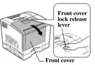
1. Grasp and pull down the **front** cover lock release lever to swing open the **front cover**.
