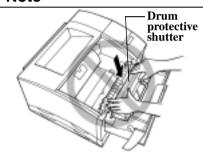
• DO NOT PRESS ON the drum protective shutter during installation. Doing so may damage the drum cartridge.
