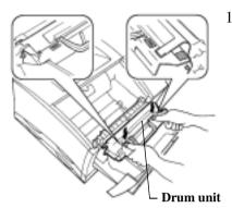
19. After clearing the misfeed, secure the **drum unit** into place by applying pressure at its top where the "**Press**" label is affixed. The **drum unit** will lock into place when it has been correctly inserted into the printer.
