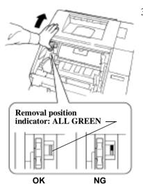
3. To confirm the rack is positioned for removing the cartridge, use the **position** confirmation window beside the dial. The **removal** position indicator will alert the user to the proper removal position.
