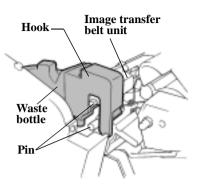
11. Make sure that the hook of the waste bottle is engaged securely by the pins of the image transfer belt unit.
