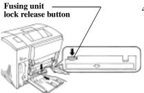
Push and hold the **fusing unit** 4. lock release button and slide out the fusing unit.
