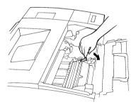
4. Return the **misfeed clearing lever** to the "down" position.
