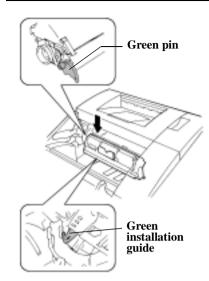
14. Insert the green pin on the left side of the cartridge into the green installation guide of the rack.
