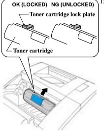
15. Firmly press the cartridge into the rack until it clicks into place.
