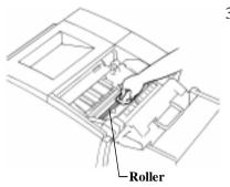
3. Using a soft cloth, wipe dirt and paper debris off the **roller** as shown.
