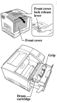
1. Grasp and pull down the **front cover lock release lever** and swing open the **front cover**.
