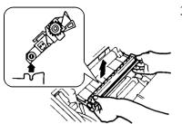
3. Pull out the **image transfer** roller unit.
