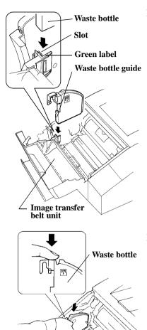
10. Slide the waste bottle into the slot located behind the image transfer belt unit on the left side of the printer. (The shape of the image transfer belt **unit** is drawn in the diagram with dash marks.)
