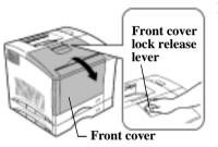
1. Grasp and pull down the **front cover lock release lever** and swing open the **front cover**.
