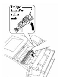
2. Lift the **image transfer roller unit** to the position shown.
