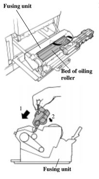
18. Remove the new **oiling roller** from its carton.
